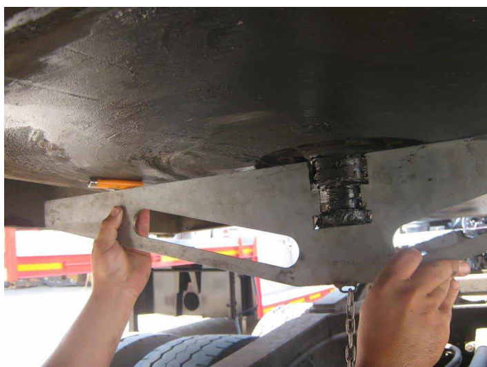
Checking for skid plate distortion
