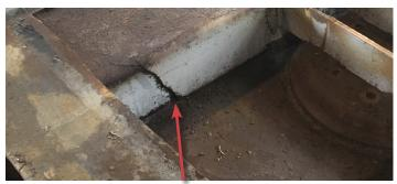
Structural cracks on a cross-member in the skid plate / king pin assembly of a refrigerated trailer (found after the flooring was removed to reveal an internal chamber).
